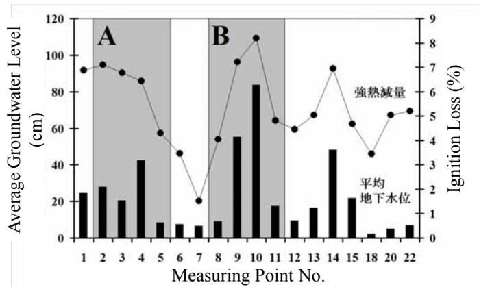
Figure 3 Distribution of Average Groundwater Level and Ignition Loss of Bedrock ( $N_c=40$ )
