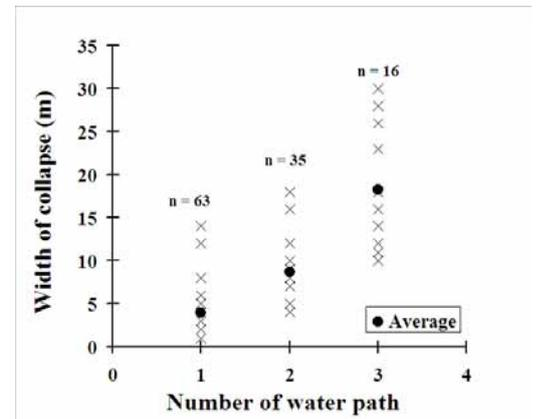
Figure 2 Relationships between The Number of Water Paths and Collapse Widths
