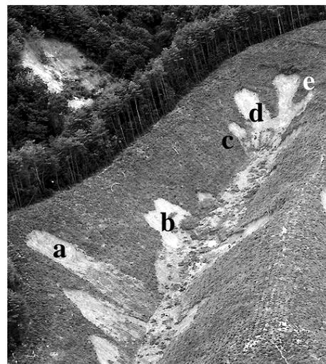
Picture 1 Case Examples of the Shapes of Shallow Landslides
