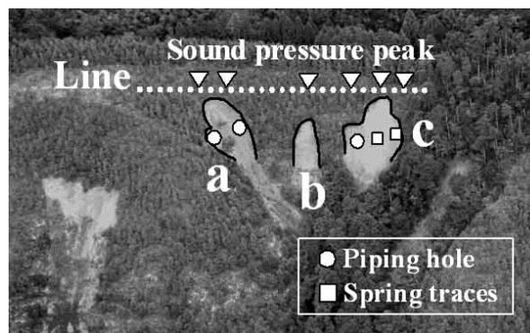
Picture 2 Shallow Landslide Occurring on a Natural Slope A
