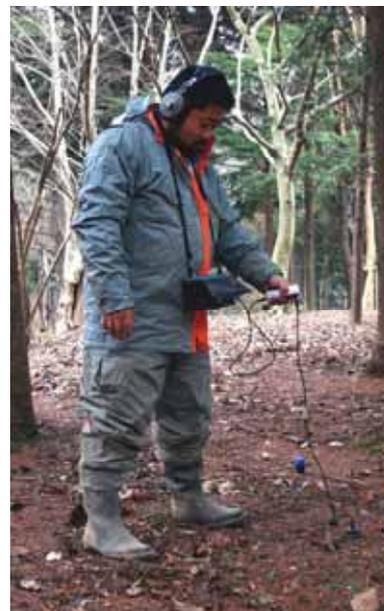
Picture-5 Showing Groundwater Aeration Sounds Being Measured
