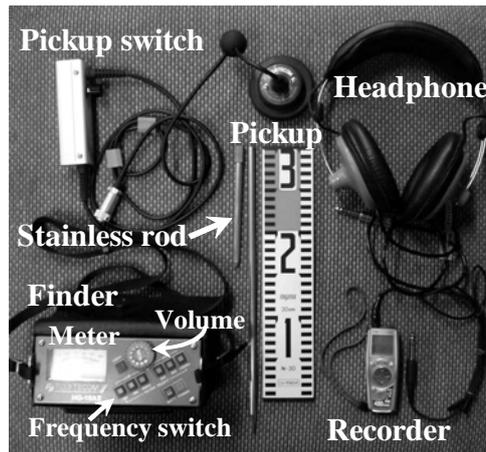
Picture-4 Groundwater Aeration Sound Measuring Device
