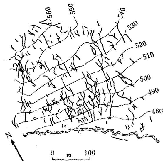
Figure-1 Networks of Underground Pipes Which Were Surveyed Using A Stethoscope (cited from Pond, S. F.(1983))
