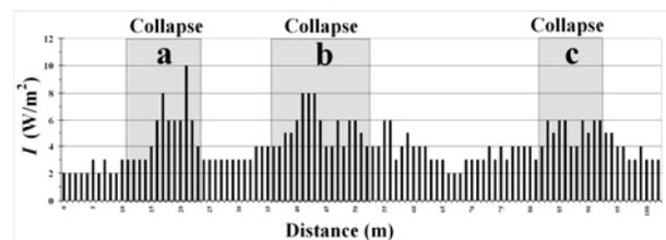
Figure-10 Distribution of Groundwater Aeration Sounds on Natural Slope C
