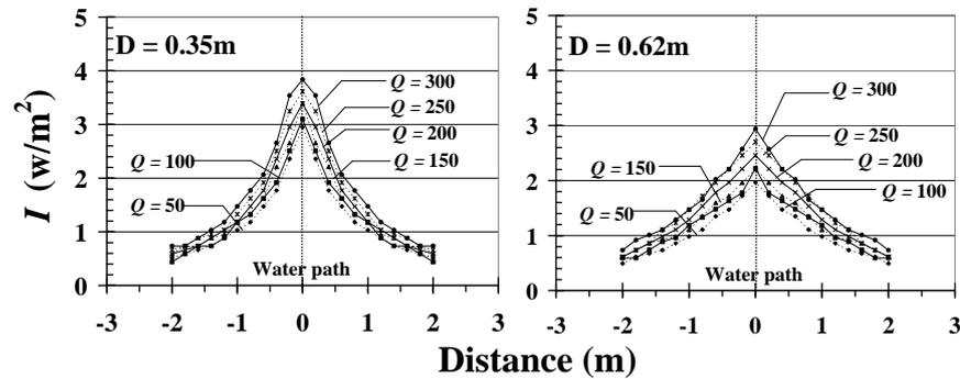
Figure-4 Results of Groundwater Aeration Sound Measurements for Each Depth
