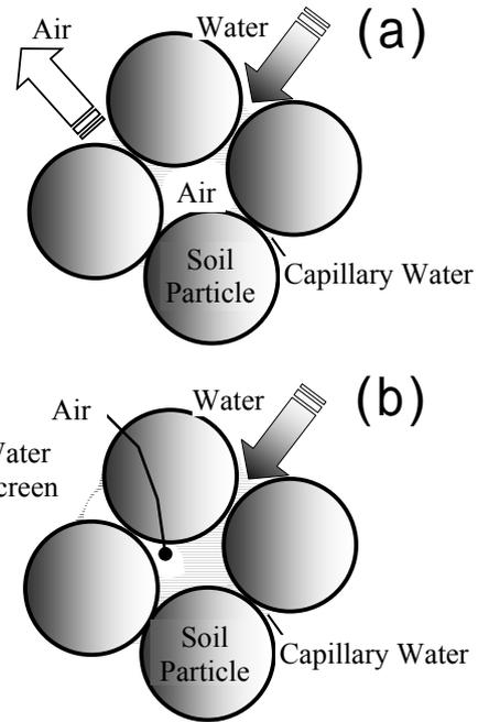
Figure-2 Movements of Water And Air in Sand Layer
